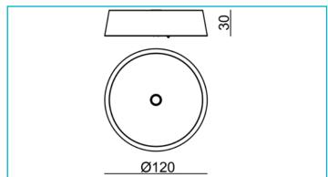
Housing Material Die-cast aluminium
