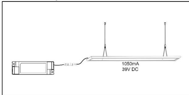
\*Do not connect the luminaire to an active LED driver. Some LED drivers emit high voltage when idle, which may cause permanent damage to the luminaire. Be sure to disconnect the LED driver from the power line before connecting the luminaire.
