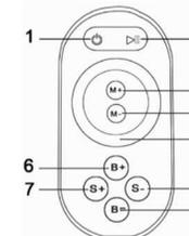
If the hand-held transmitter is not used for longer than 20 seconds, it automatically switches into the standby-modus. By slightly shaking it is ready for operation again.
