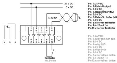
Dreidrahttechnik/three wire circuit
